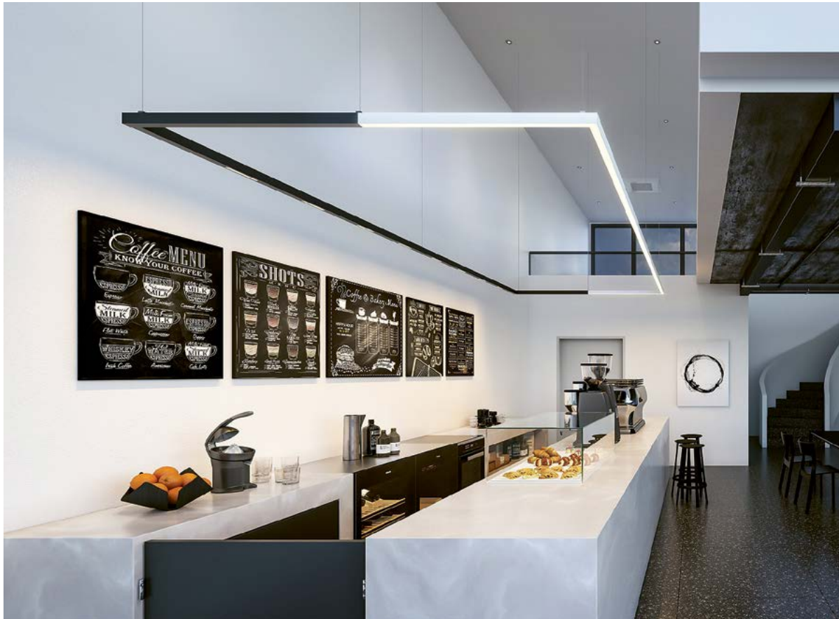
MILUM Lightline mit Diffusor opal; in Kombination mit MILUM Wallwasher-Modulen MILUM lightline with opal diffuser; combined with MILUM wallwasher modules
